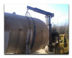
ITS is more diversified to handle the most strategic projects with our three Vera-Lifts. Our 60/80 lift with boom has a lifting capacity of 100,000 lbs. The 40/60 has a 60,000 lb lifting capacity with a boom that reaches a height of 26 ft. and our 25/35 can lift 35,000 lbs. and is equipped with a three section boom that reaches 23 ft.
